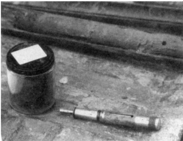
Figure 3-9 Field SPT sampling sequence. (a) Split tube opened to display sample and for taking a pocket penetrometer test for q_u . (b) Placing representative sample into jar for laboratory use. (c) Sample in jar with identification label. Pocket penetrometer in foreground. Dark band is marker for q_u on calibrated stem.
