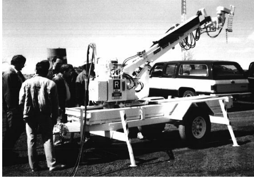
Figure 15.7: Compact trailer-mounted robot unit for remote controlled shotcrete application.
