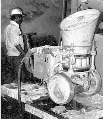
Typical dry mix shotcrete machine.
