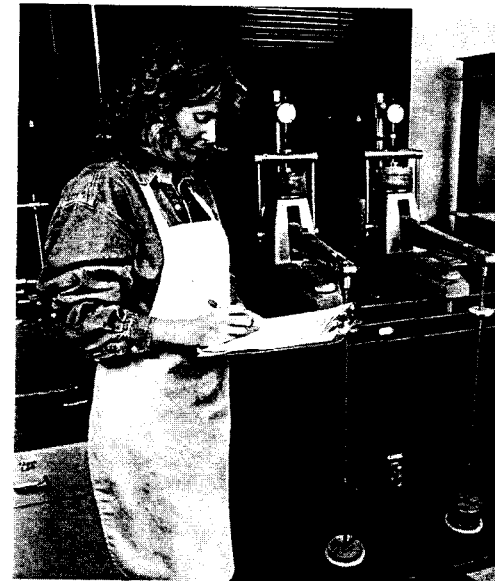
Figure 3.6 (a) Performing consolidation tests in the laboratory. The two consolidometers use the weights in the foreground to load the samples; (b) cross section of a consolidometer.
