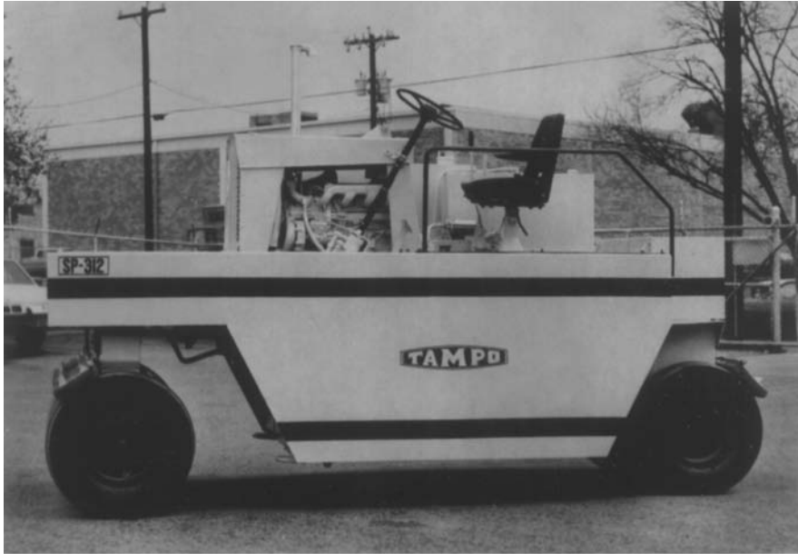
Figure 14.3 Pneumatic rubber-tired roller (Courtesy of Tampro Manufacturing Co., Inc., San Antonio, Texas)
