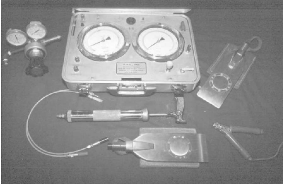
Figure 2.35 Dilatometer and other equipment (Courtesy of N. Sivakugan, James Cook University, Australia)
