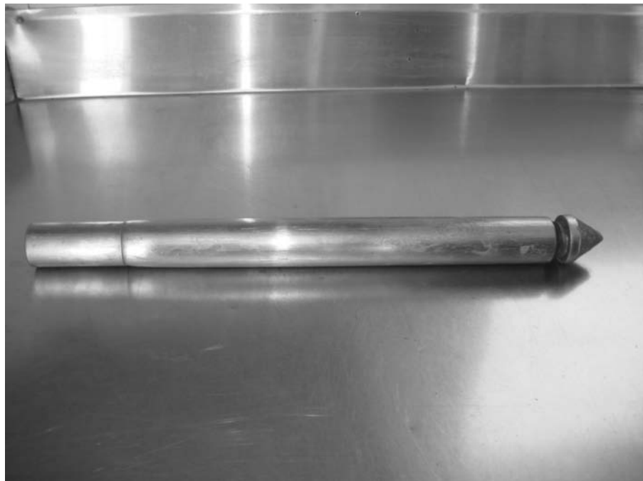
Figure 2.25 Photograph of an electric friction-cone penetrometer (Courtesy of Sanjeev Kumar, Southern Illinois University, Carbondale, Illinois)
