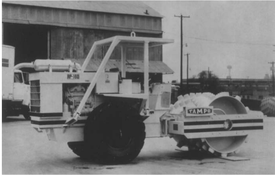
Figure 14.4 Vibratory sheepfoot roller (Courtesy of Tampro Manufacturing Co., Inc., San Antonio, Texas)
