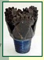
Drilling: Rotary Bit
