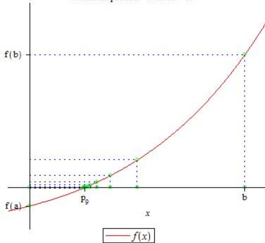
10 iteration(s) of the method of false position applied to
