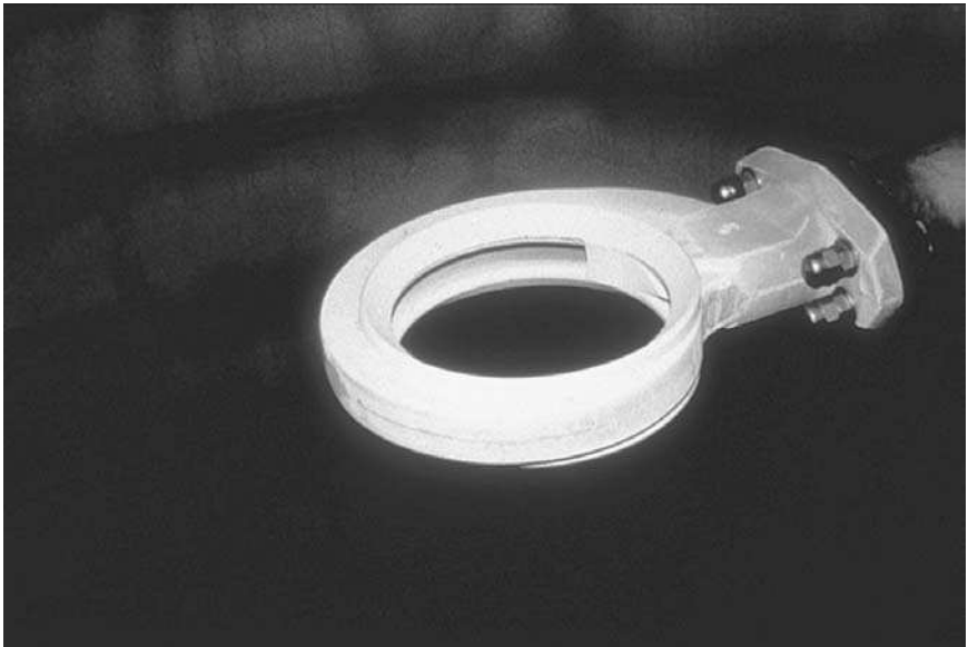
FIGURE 11.2.4 Absorber vessel spray nozzle.
