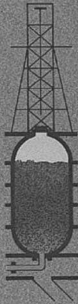
FIGURE 12.1.7 Coke drum drilling cycle, based upon a 24-h drum fill cycle operation.
