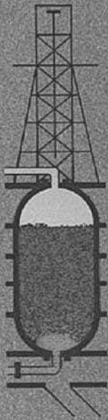
FIGURE 12.1.7 Coke drum drilling cycle, based upon a 24-h drum fill cycle operation.
