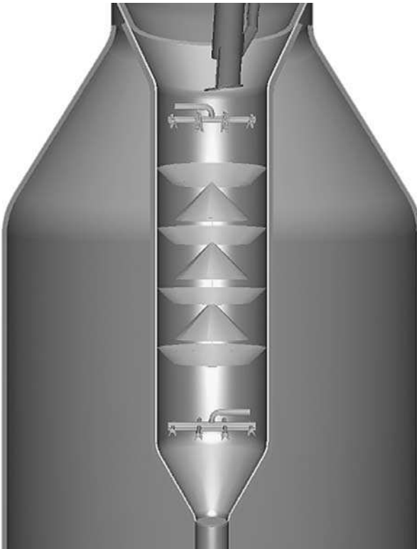
FIGURE 3.1.7 Spent catalyst stripper.
