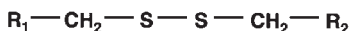
FIGURE 8.1.2 Typical petroleum molecules that contain sulfur atoms. Sulfur atoms usually have simple chemical bonds in petroleum.
