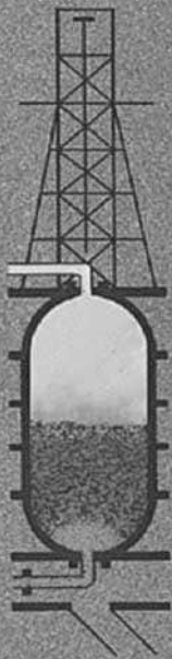
FIGURE 12.1.7 Coke drum drilling cycle, based upon a 24-h drum fill cycle operation.
