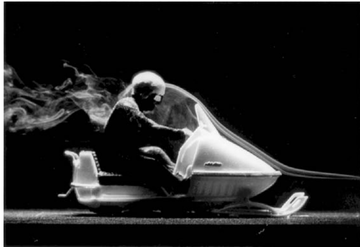
PLATE 2 Flow around a snowmobile. (Photograph courtesy of the National Research Council of Canada.)
