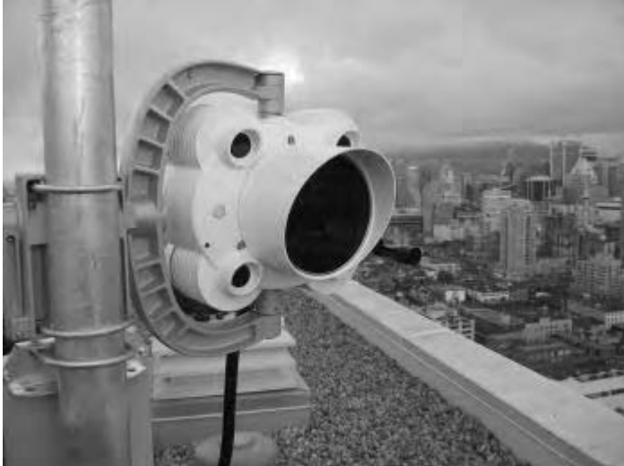
Figure 24-24 A rooftop, free-space optics system operates in the skies over Vancouver, BC, Canada. (Source: fSONA Systems.)
