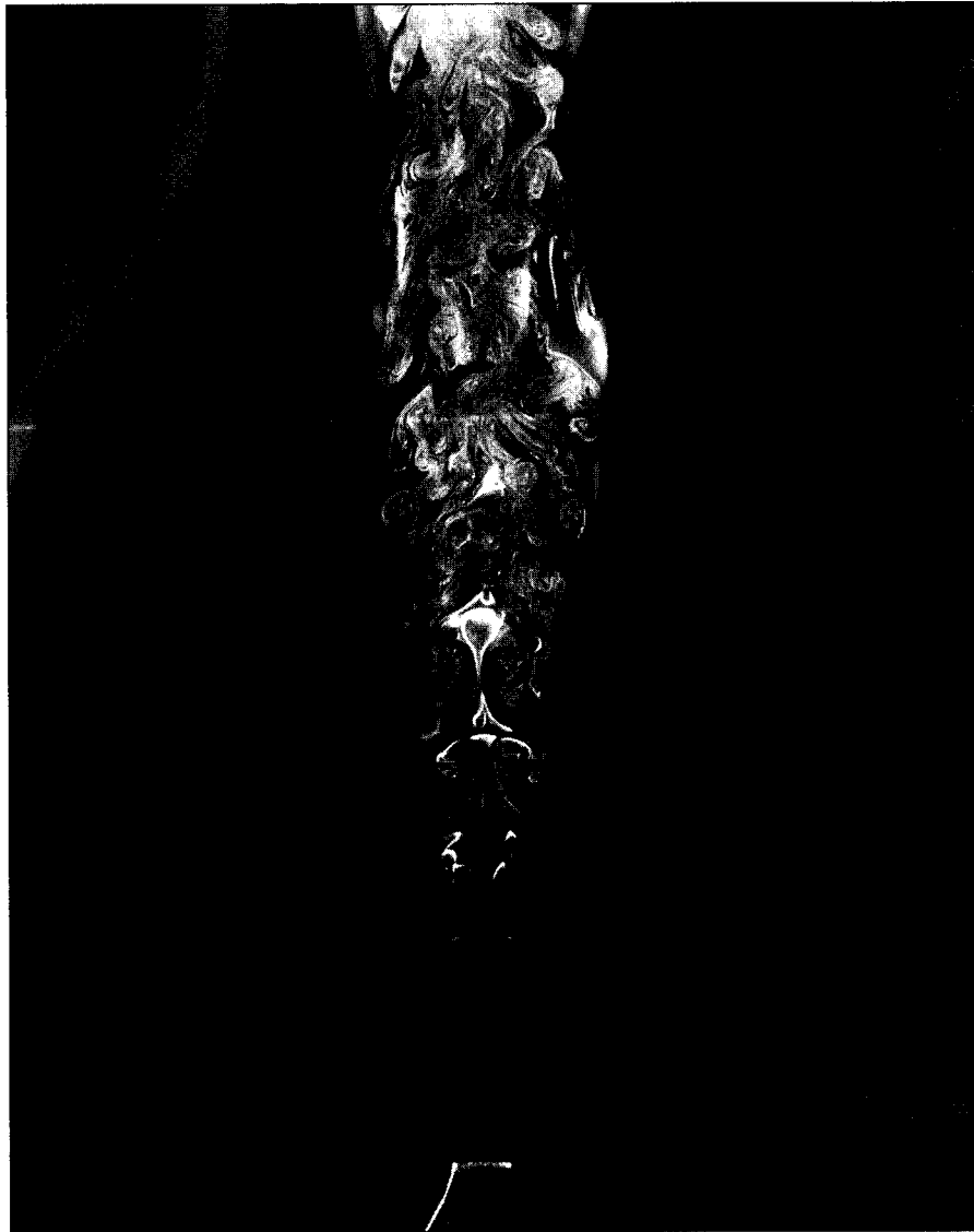
Figure 13.6 Visualization of nozzle-fluid flow patterns using reactive Mie scattering in methane-air jet flame ( v_e = 10 m/s, d_j = 10 mm). The total length of the image is approximately 20 nozzle-diameters. Near the nozzle, the flame zone resides just outside of the rollup of the nozzle shear layer. Near the top of the photograph, the flame zone interacts with the turbulent core. The visualization of an outer layer results from water vapor from the flame reacting with \text{TiCl}_4 vapor in the surrounding air flow. | SOURCE: Photograph courtesy of W. M. Roquemore. See also Ref. [7].
