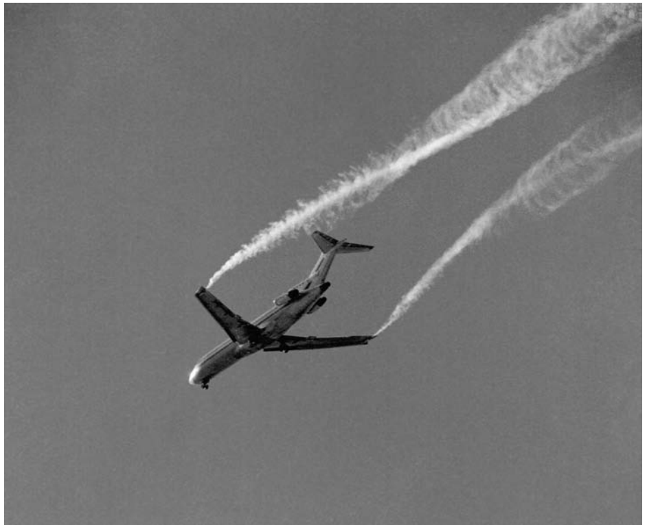
Fig. 8.28 Wingtip vortices from a smoke-visualization test of a Boeing 737. Vortices from large airplanes can be extremely dangerous to any following aircraft, especially small planes. This test was part of a research effort to alleviate these swirling wakes. (NASA photo.)
