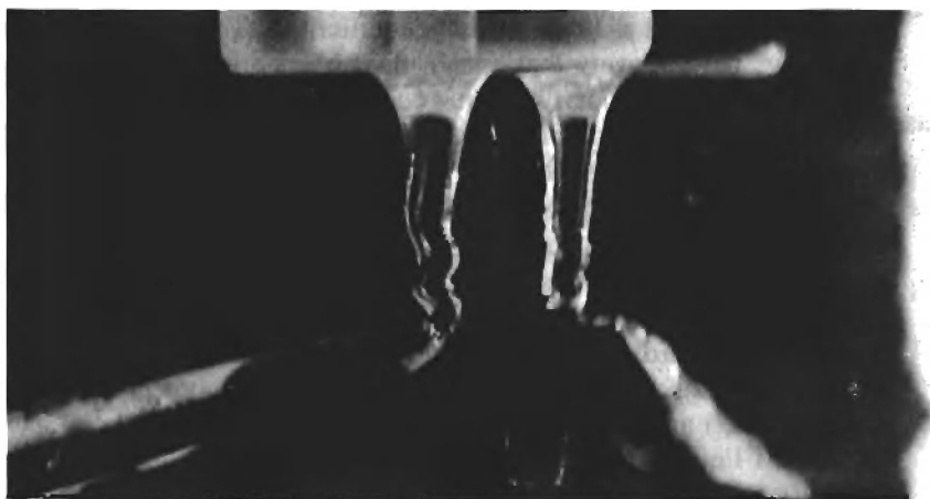
Figure 6.4 Plane buckled shape of a water column impinging on the flat end of a screwdriver: left side, direct view; right side, view through the side mirror. (From Ref. 26.)
