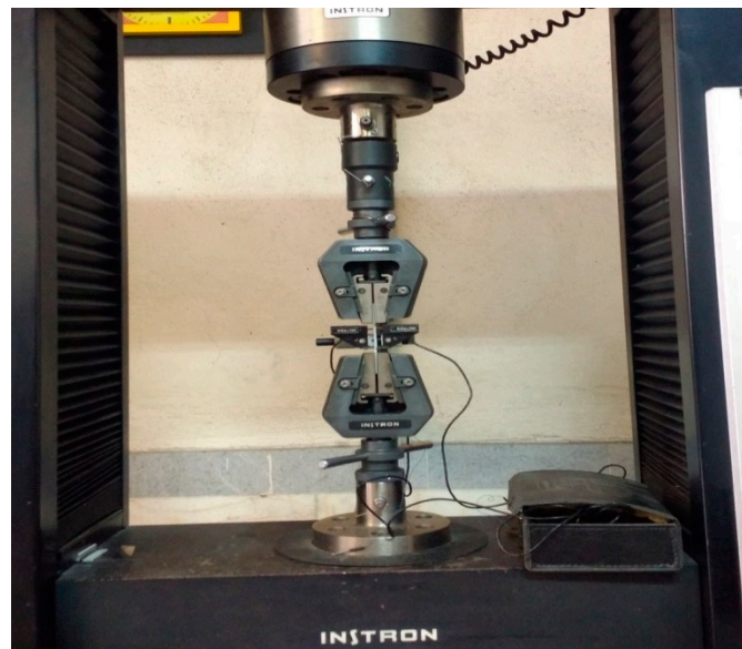
Figure 1. Uniaxial tensile test.
