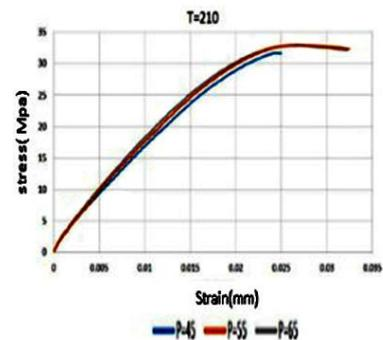
Figure 19. stress- strain diagram of ABS polymer in the temperature of 210 centigrade and pressures of 45 and 55 and 65 MPa
