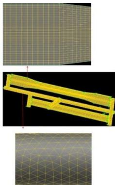
Figure 3. The mold geometry which is meshed by Gambit
