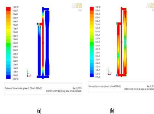
**Figure 10.** a) Filling the mold in (a) 0.2 and (b) in 0.4 seconds in temperature of 190 and pressure of 65
