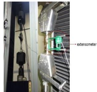
Figure 7. Tensile test machine and extensometer
