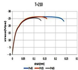
Figure 17. stress- strain diagram for PP at 210°C in different pressures
