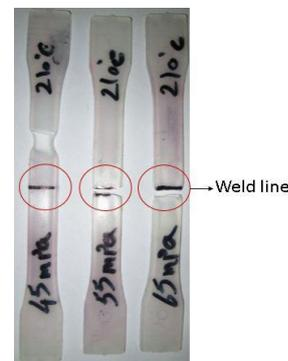
**Figure 16.** Weld line and fracture locations for the PP samples produced by different injection pressures at 210°C
