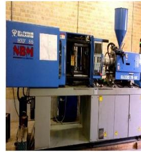
Figure 4. plastic injection machine
