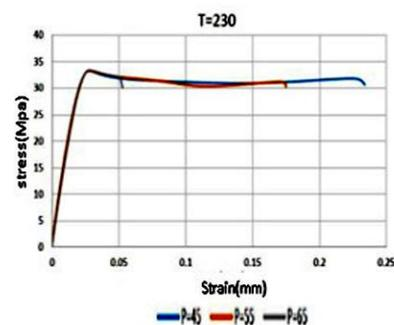
Figure 20. stress-strain diagram of ABS polymer in the temperature of 230 centigrade and in pressures of 45 and 55 and 65 MPa
