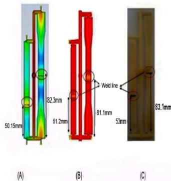
**Figure 8.** Weld line location (comparison between numerical models and the experiment) A) Result of Mold Flow, B) Result of FLUENT, C) Result of the performed experiment
