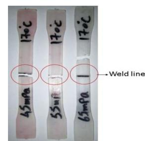
**Figure 11.** Weld line and fracture line locations for the PP samples produced by different injection pressures at 170°C
