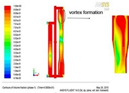
**Figure 12.** Formation of vortex in PP melt at injection pressure of 65 MPa and injection temperature of 170°C
