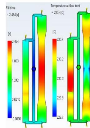
**Figure 9.** a) mold filling time of ABS, b) temperature distribution of ABS melt front (Results of Mold Flow)
