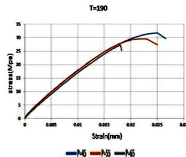
Figure 18. Stress- strain of ABS polymer in the temperature of 190 centigrade and in pressures of 45 and 55 and 65 MPa
