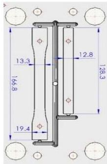
Figure 2. The mold geometry (dimensions, mm)
