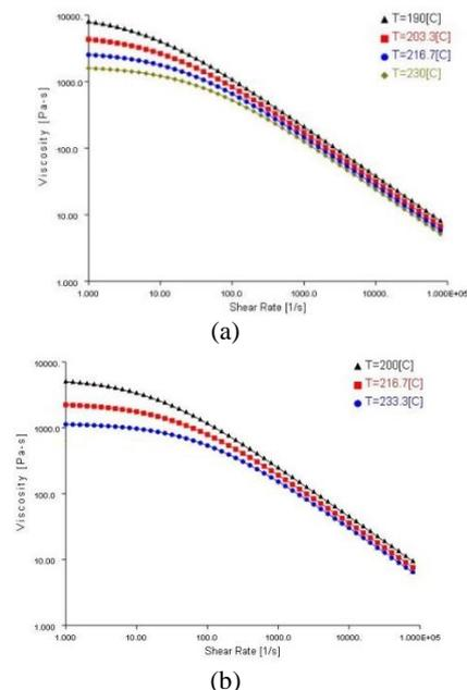
**Figure 1.** Variation of viscosity against shear rate for a) PP, b) ABS
