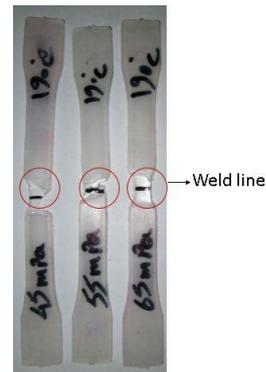
**Figure 15.** Weld line and fracture locations for the PP samples produced by different injection pressures at 190°C
