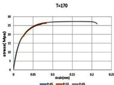
**Figure 14.** stress- strain diagram for PP at 170°C in different pressures
