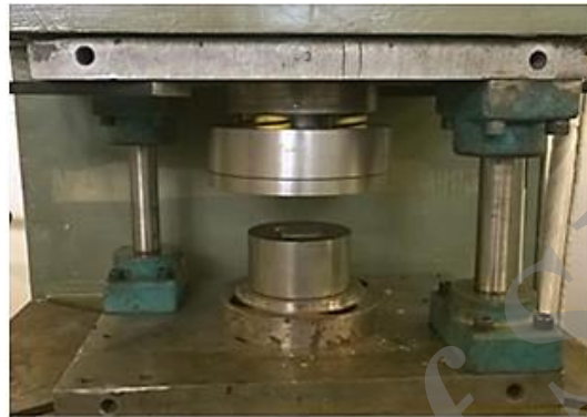
Fig. 6. Deep drawing die used in experiments.
