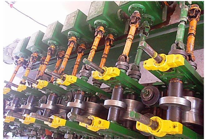
Fig. 3. Cold roll forming line.
