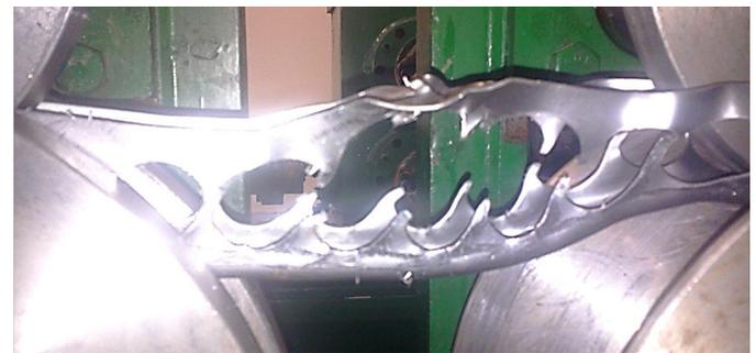
Fig. 14. Sample failure resulting from hole spacing that was too tight.
