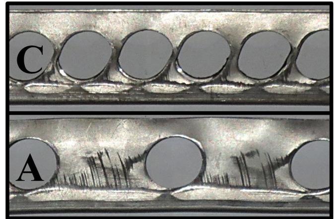
Fig. 13. Transition from type C to type A ovality with increasing hole spacing.
