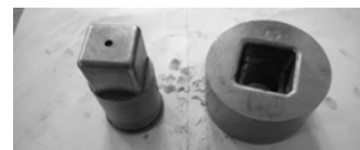
Fig. 2 Punch and matrix experimental test
