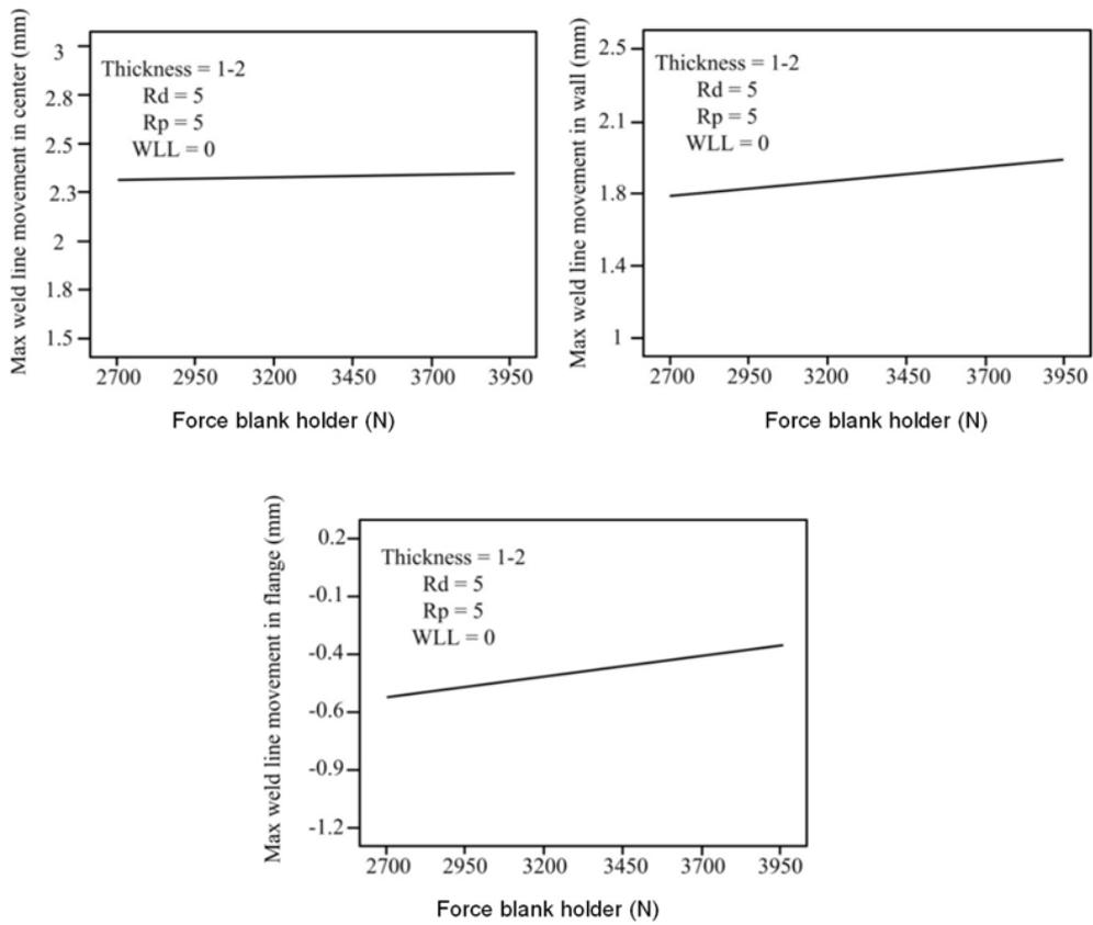
Fig. 11. The effect of weld line location on its movement.
