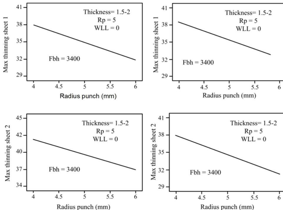
Fig. 8. The effect of punch and die's radius, on the percentage of sheet 1 and 2 thinning.
