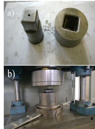
**Fig. 2.** a) Punch and die of the experimental test, b) Experimental test set.
