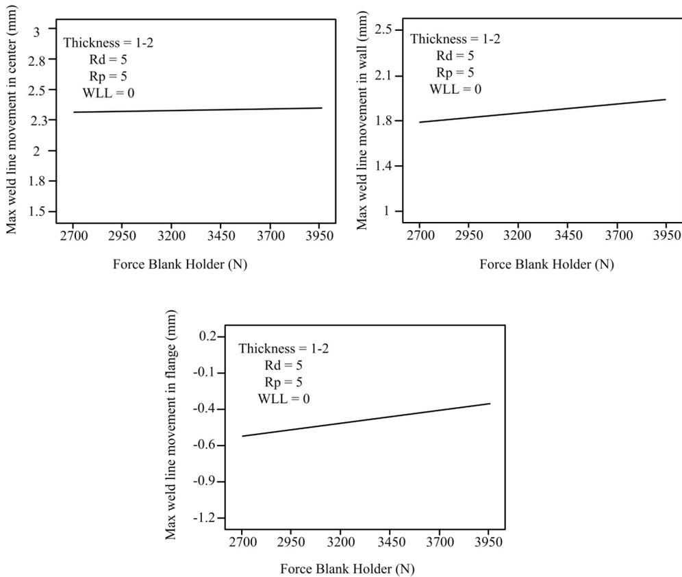
Fig. 12. The effect of blank holder force, on the weld line movement.
