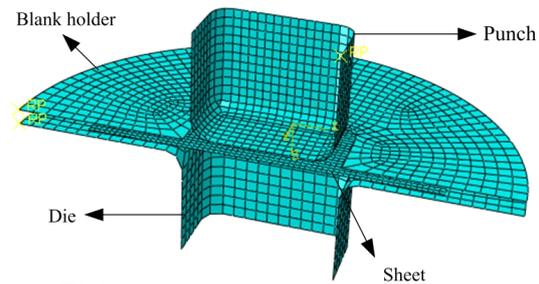
**Fig. 4.** Finite element model.
