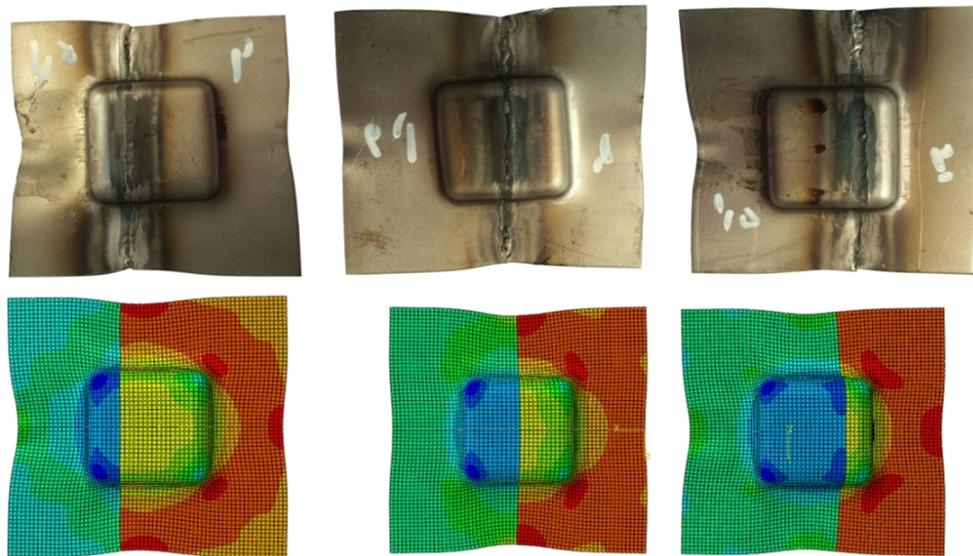
**Fig. 7.** Simulation and experimental results of weld line movement.
