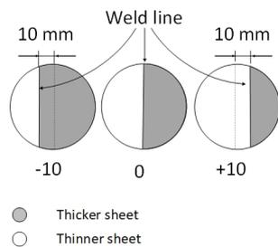
**Fig. 1.** Tailor-welded blank lay-out.
