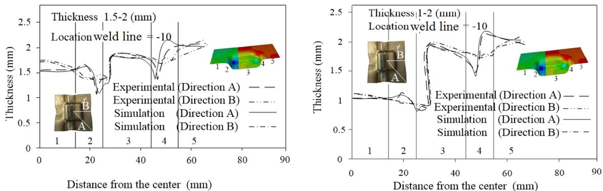
**Fig. 6.** Experimental and numerical results of thinning, in thickness combination of  $1.5\text{-}2\text{mm}$ ,  $1\text{-}2\text{mm}$ , location weld line  $-10$ .
