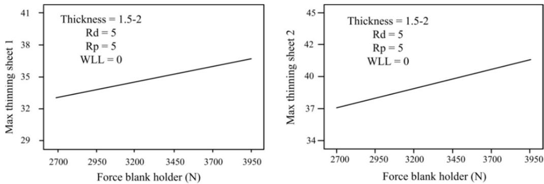
Fig. 9. The effect of the force of blank holder, on the percentage of thinning.
