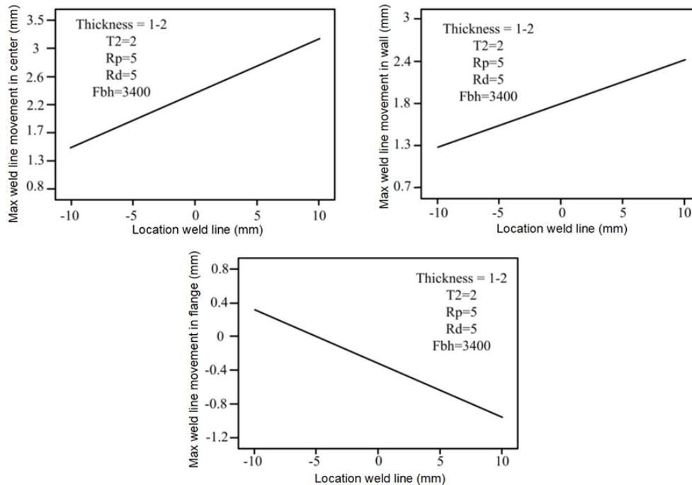
Fig. 10. The effect of punch radius on weld line movement.
