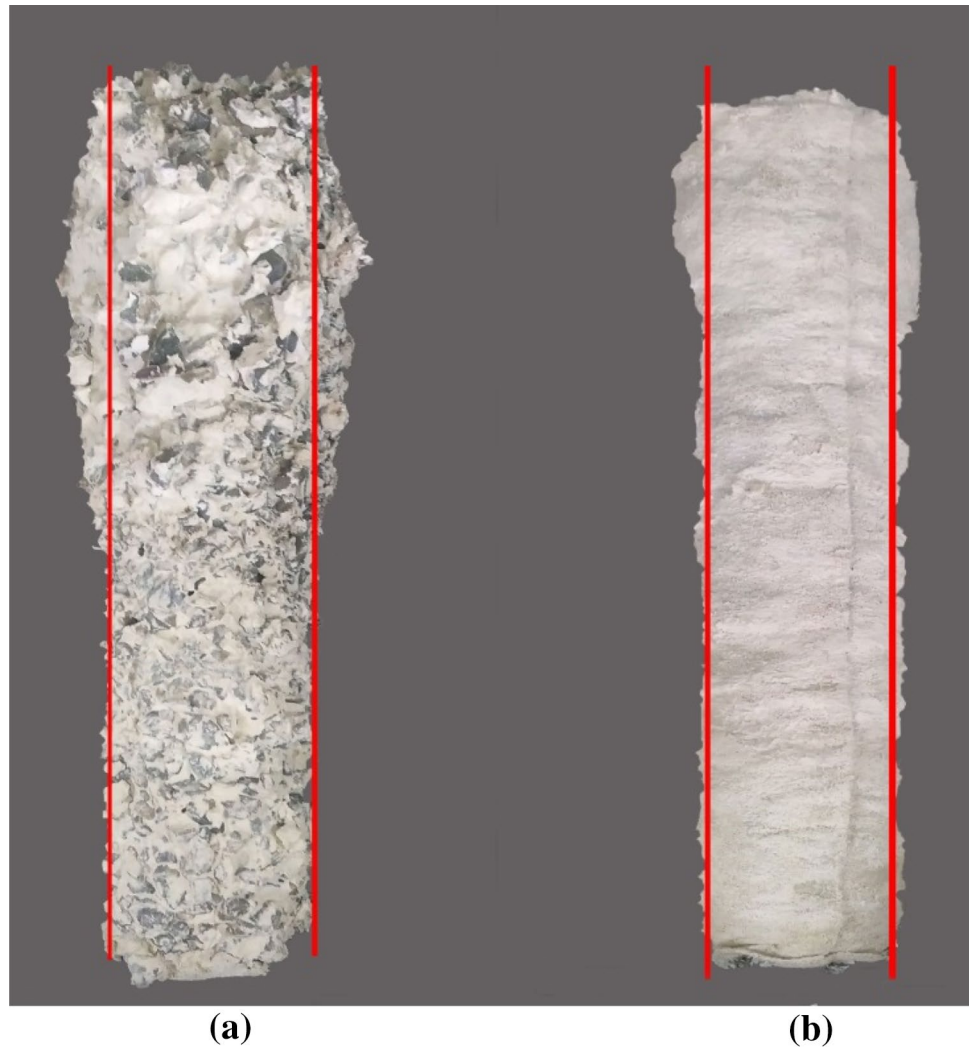
Fig. 9 Deformation of columns after test: a OSC, b VESC
